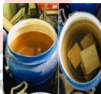
**Acid Attack test:** This test was done after the curing of specimens(cubes) for 28 days and the specimens were dried for 1 day then again were immersed in water with 5% dilution in Hydrochloric acid for 56 days and 90 days and there compressive tests and weight reduction tests were conducted.
