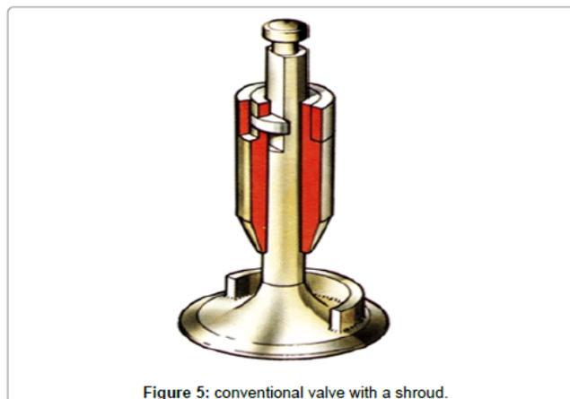
**Figure 5:** conventional valve with a shroud.
