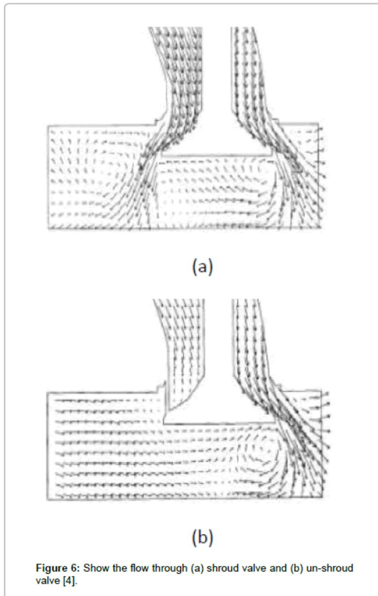
**Figure 6:** Show the flow through (a) shroud valve and (b) un-shroud valve [4].
