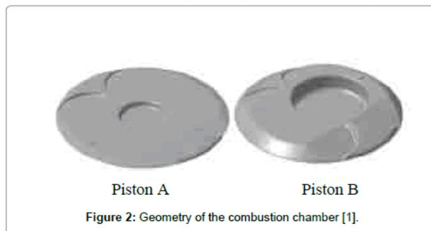
Figure 2: Geometry of the combustion chamber [1].
