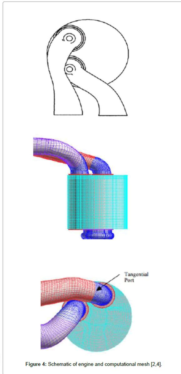
**Figure 4:** Schematic of engine and computational mesh [2,4].
