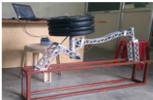
Figure 5.2: Experimental testing setup for vertical loading test
