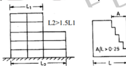
Figure 01 - Concept of Vertical Geometric Irregularity from IS 1893:2002[12]
