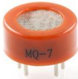
Fig -3: Gas Sensor
