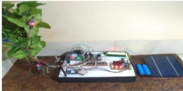
In this system we have used multiple sensors like pH sensor, fire sensor, accelerometer, ultrasonic sensor. The block diagram of various contents are as follows:
