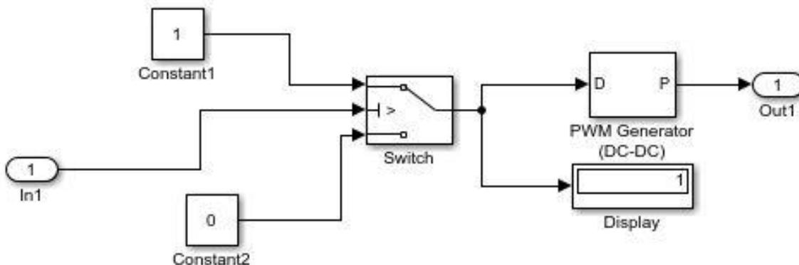
Fig. 5 Simulink model of control logic
