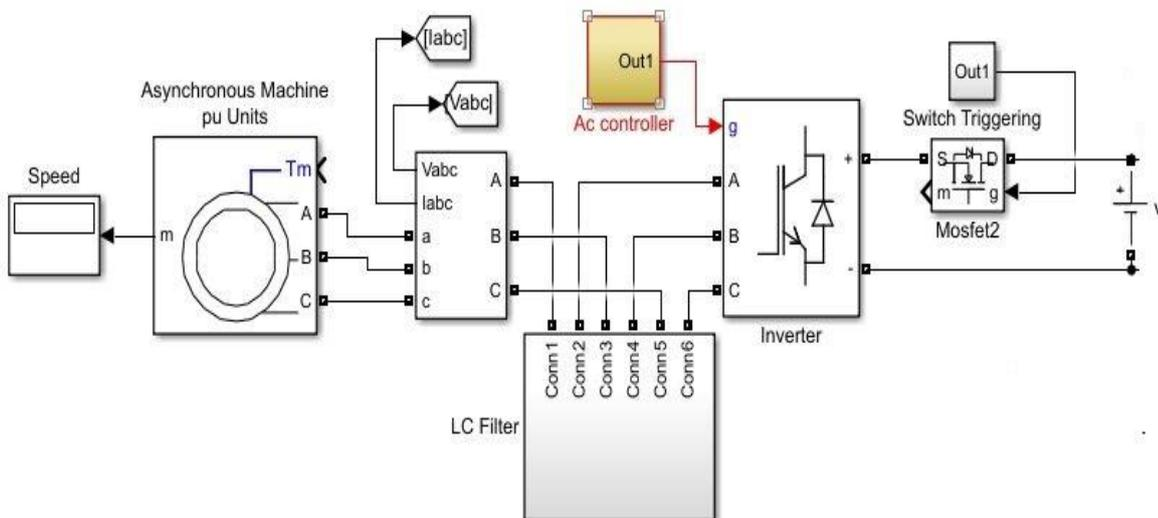
Fig. 3 Simulink model of VSG
