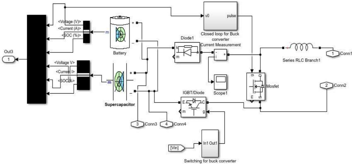
Fig. 4 Simulink model of DC voltage controller
