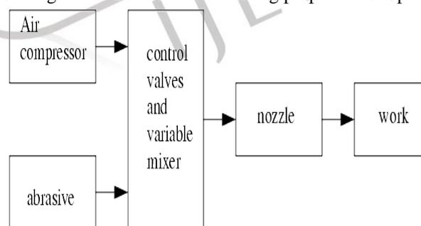
Fig 1: Line Diagram of Abrasive Jet Machining Process
