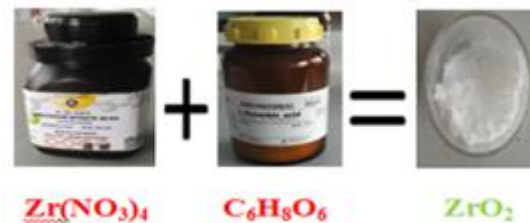
Figure 1: Sequences of procedure for preparation of ZrO 2 nano particles by the solution combustion process
