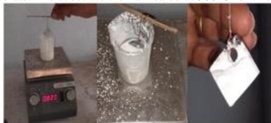
Figure 3: Coating sequence of TiO 2 nanoparticles on mild steel
