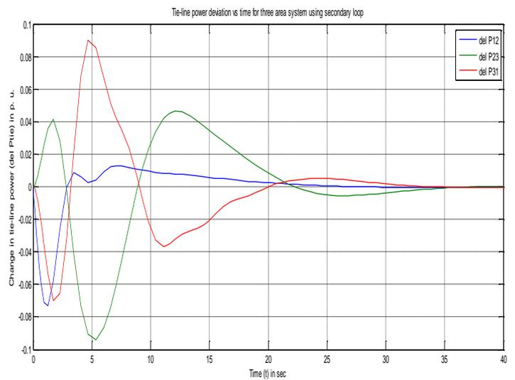
Fig 6: Tie-line power deviation vs time using IBFOA
