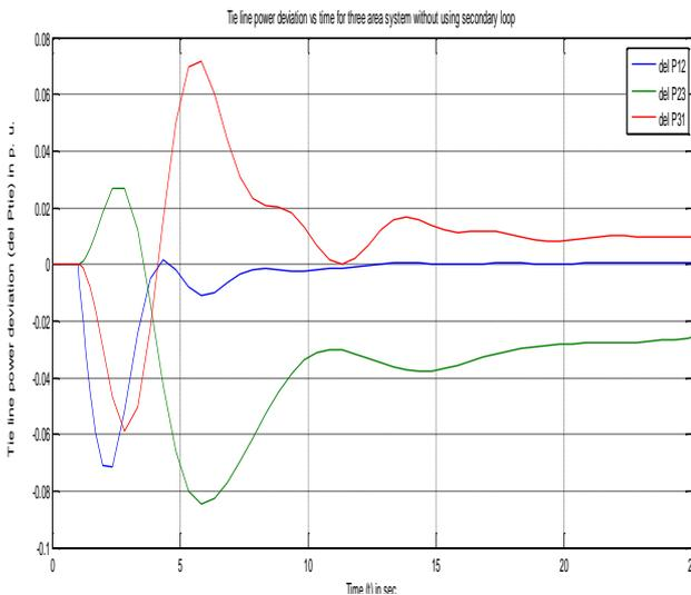
Fig 5: Tie-line power deviation vs time using PI controllers
