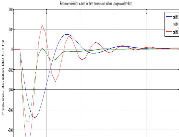
Fig 3: Frequency Deviation vs time using PI controllers
