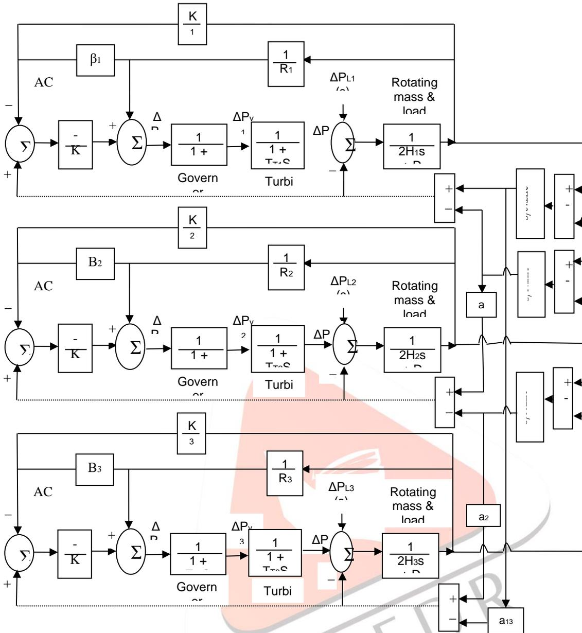
Fig 2: Three area power system by using secondary LFC loop
