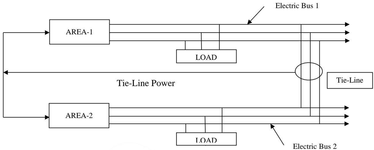
Fig1: Conventional Two Area System: Basic Block Diagram
