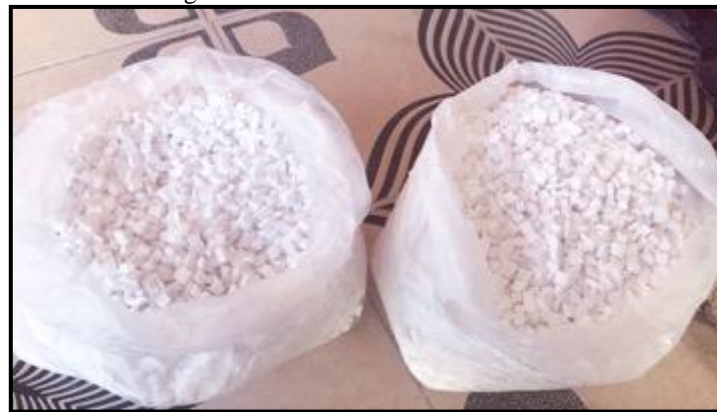
Figure 2 Recycled EPS aggregate used in concrete mixtures
