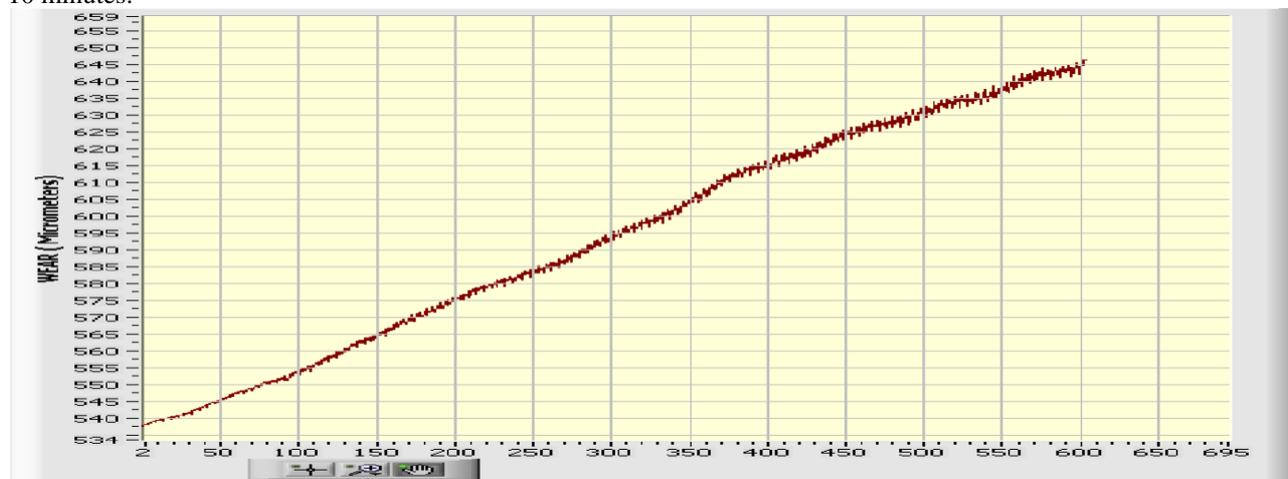
Fig- Wear at load 5 KN
