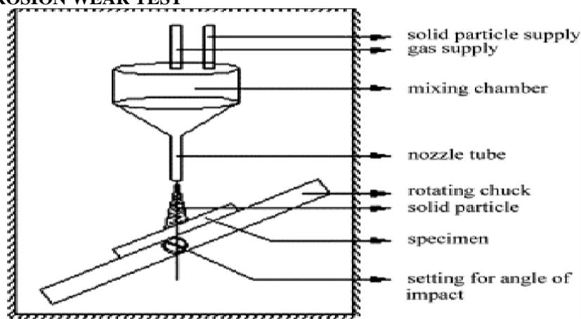
Fig. Erosion wear test apparatus
