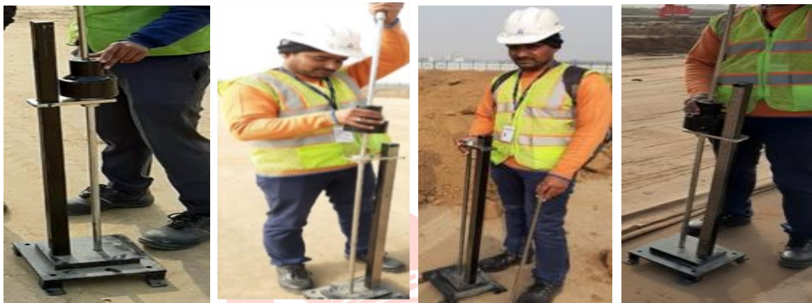
Fig.6: Dynamic Cone Penetrometer Set-up in the field
