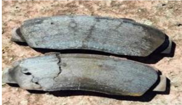
Figure 1. Brake Pad crack View
