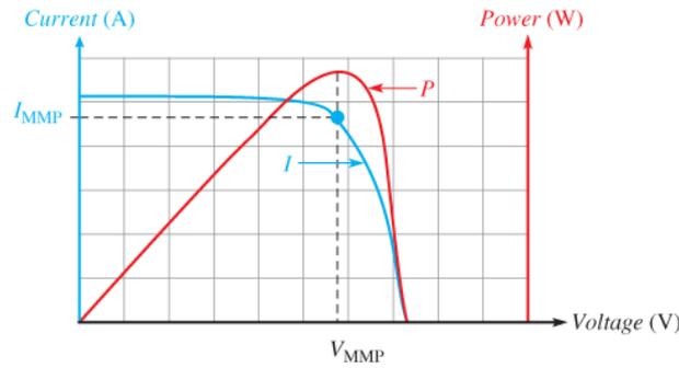
The above figure shows maximum powerpoint. There is only point in the IV\_characteristics of PV module at which power delivered by PV module is maximum. The MPPT and charge controller are two different functions, The developer combined this two function in one electrical circuitry called MPPT charge controller.
