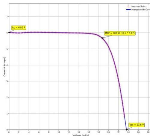
Fig.4 Graphical Representation of Automatic IV Tracer
