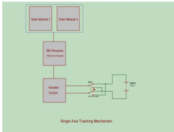
Fig.3 Single Axis Tracking Mechanism
