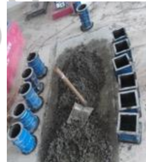
(C) Filling of Moulds
