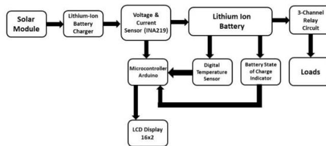
**Figure2: Block diagram of BMS**
