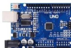
Arduino is an open-source gadgets which is easy to utilizing and programming. Arduino Uno has total 14 pins, from which 6 pins provide PWM output and 6 pins provides analog inputs. Instructions as well as programming is fed through portable drive. For this you can use the programming language and the Software (IDE) arguing.
