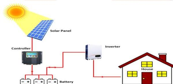
**Figure 1: Diagram of complete solar PV energy system**
