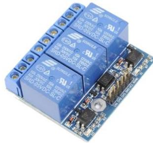
In this project, three channel relay circuit will be implemented, which will be used to control the load based on battery state of charge. Loads will be made ON and OFF based on the priority.
