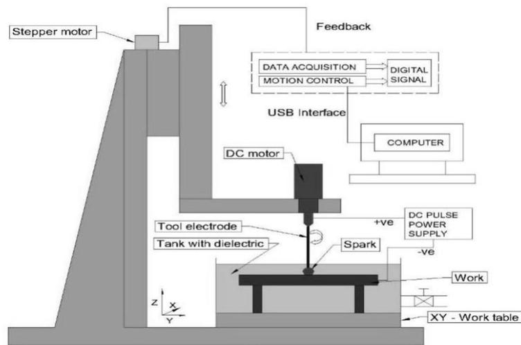
Fig 1.1 Schematic of micro-EDM set-up<sub>1</sub>
