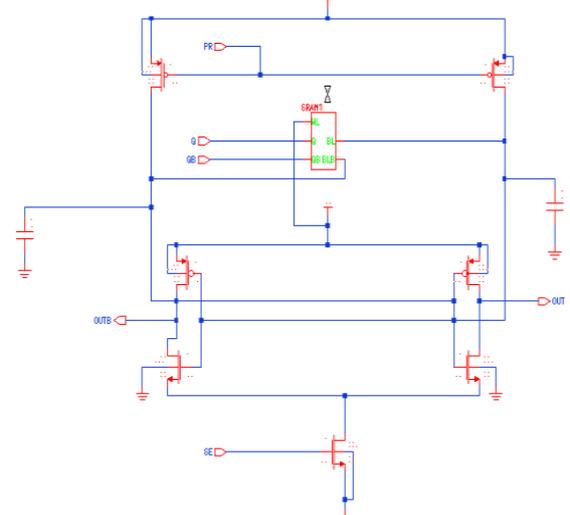
**Figure 2 Cross coupled CMOS inverter SA**
