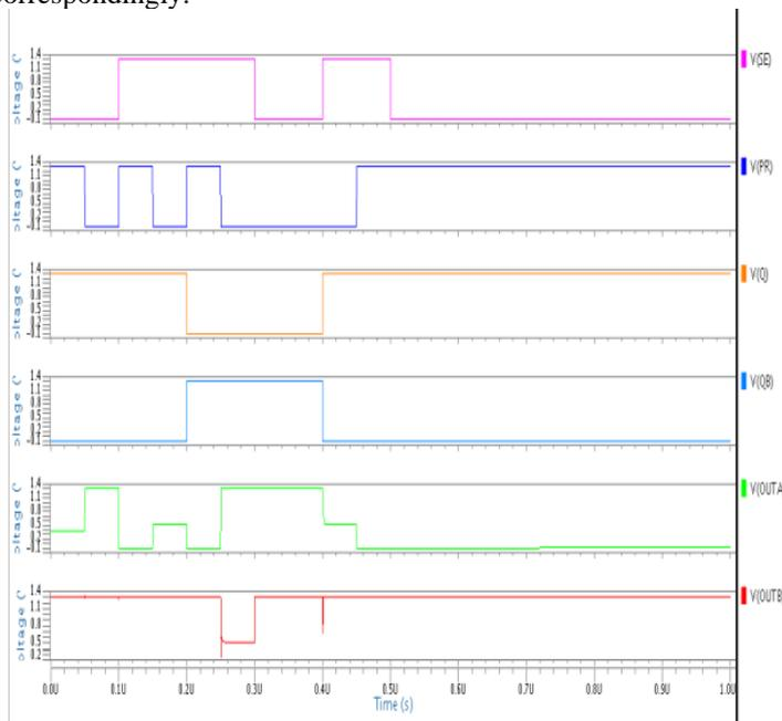
Figure 6 Reading operation in Latch type SA
