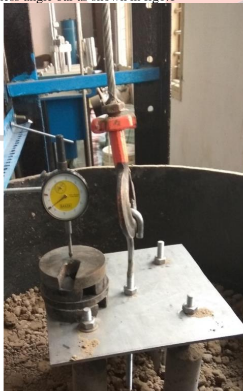
Fig3.2.3 showing the placement of dial gauge on group pile.
