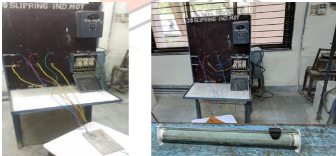
Figure 9 Hardware Setup of Slip-Ring Induction Motor with External Resistance (Rheostat)
