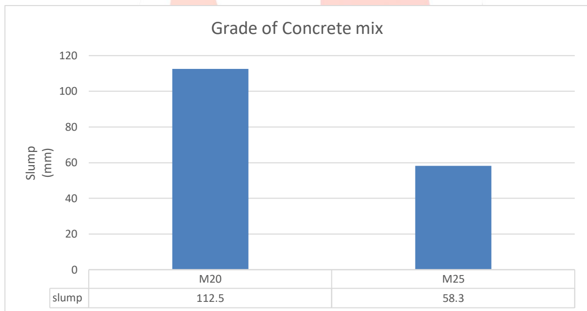
Figure 3. – average slump height on addition of percentage of plastic (5%, 7.5%, 10%, 12.5%, 15%) in M20 and M25 grade of concrete.
