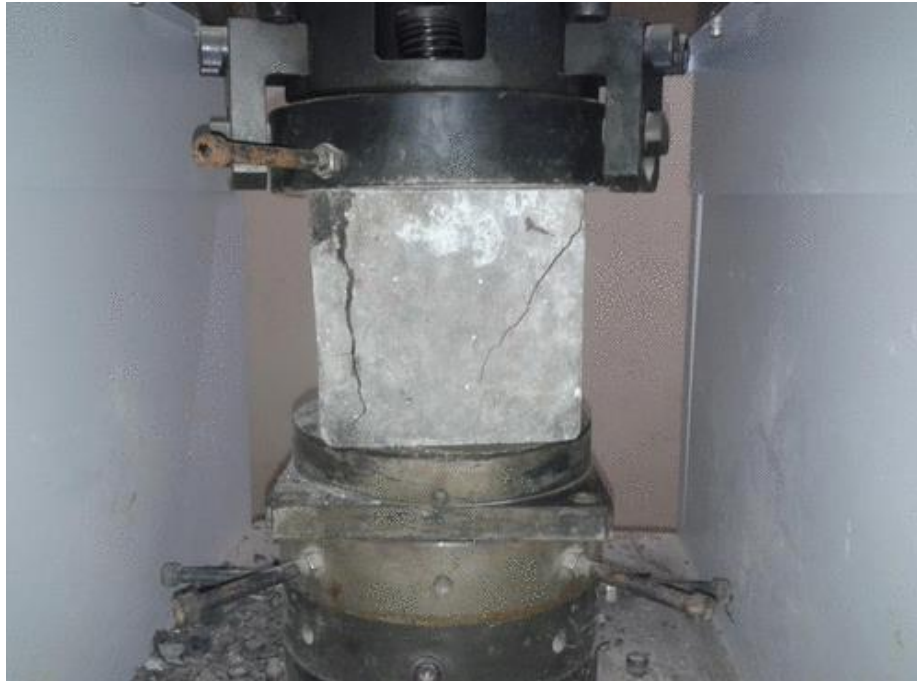
Figure 4. – Concrete subjected to loading
