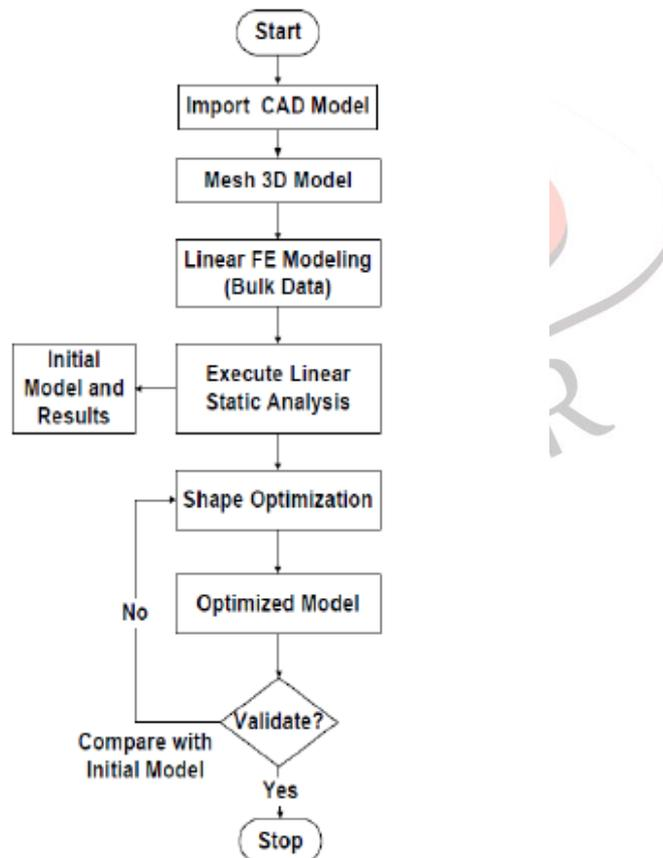
**Fig 2: Design Methodology Process Flowchart**
