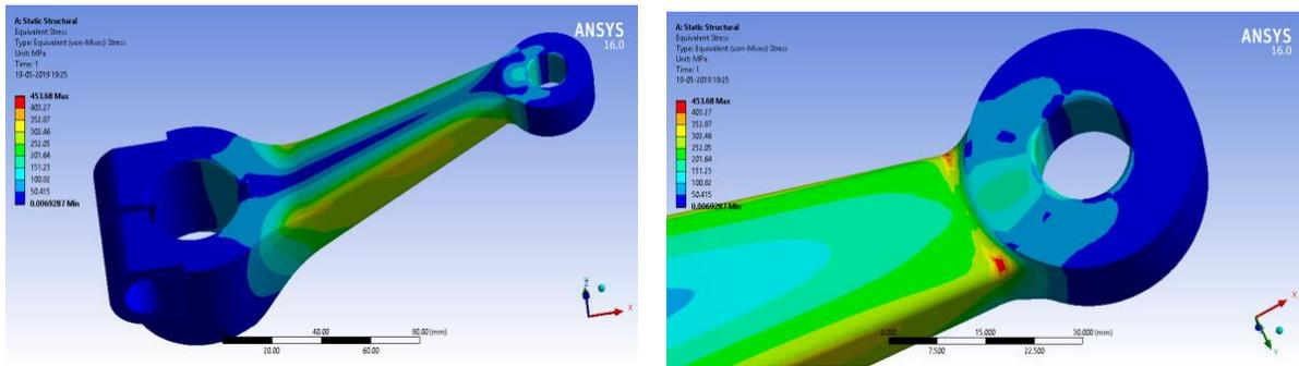
**Fig 6:** Static analysis results of steering arm using SAE 1045, von-mises stress in steering arm is 453.68 N/mm<sup>2</sup>.
