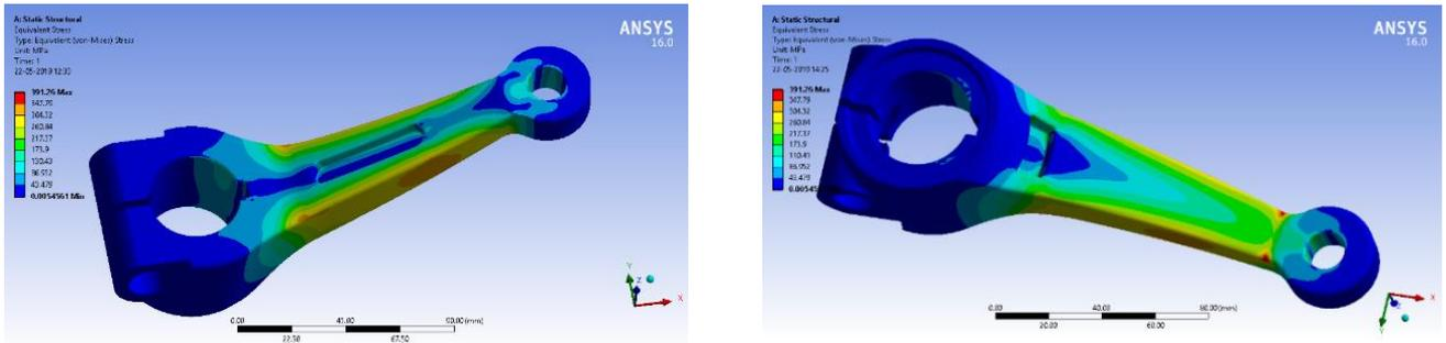
**Fig.8.** Stress contour of modified model
