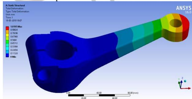
**Fig.5. Displacement Contour**
