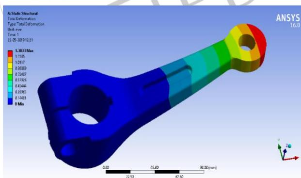
**Fig.7.** Displacement contour of modified model
