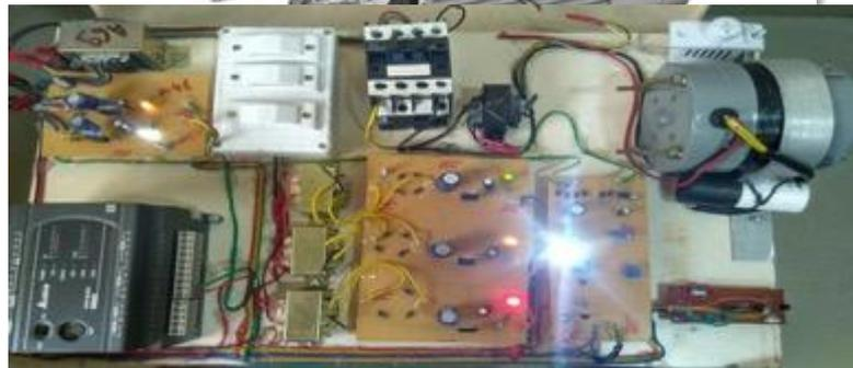
In this automatic fault detection and protection system, three phase auto-transformer is employed to offer the availability voltage to the induction motor. to scale back the voltage level there's potential divider circuitry is applied and input required to PLC should be DC. Hence there's rectifier circuit is employed to convert AC to DC. Switches are connected in between the lines to make the manual fault which are Line-to-Line.
