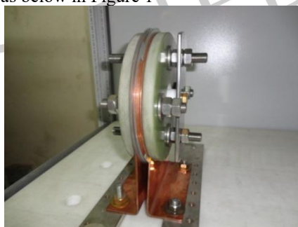
Figure 1.1 complete assembly of helical disc based coil
