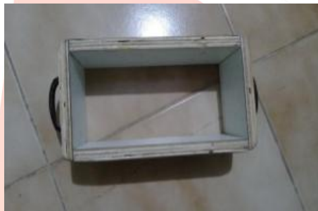
Fig 4.5 Standard brick mould
