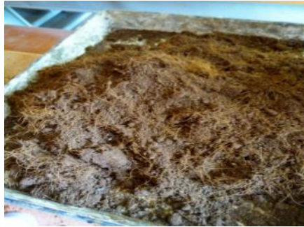
Fig 4.4 Wet mix of soil cement and fibers
