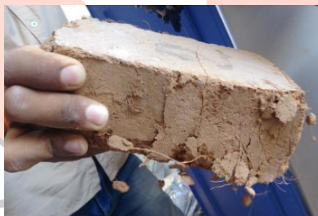
Fig 5 Failure of the bricks
