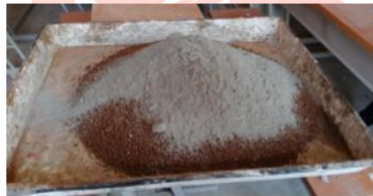
Fig 4.2 Mixing of soil and cement
