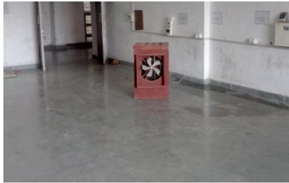
Fig. 3 Actual View of Clay tube Air cooler placed in room
