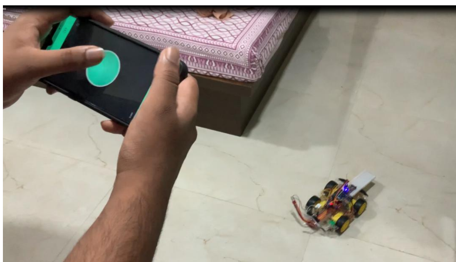
Figure 4.3 Robot Controlling using BLYNK Application
