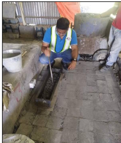
Fig. 5 Compaction of Concrete Beam in Concrete Lab
