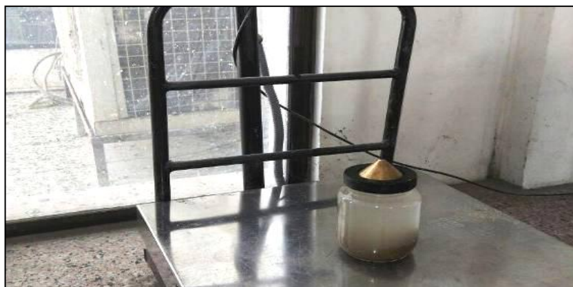
Fig. 1 Determination Specific Gravity of Aggregates by Pycnometer
