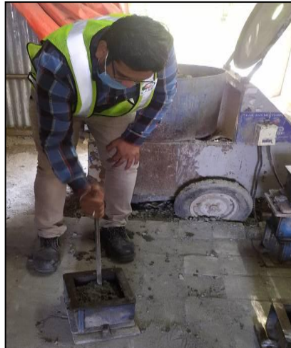
Fig.4 Compaction of Concrete Cube by Tamping In Concrete Lab
