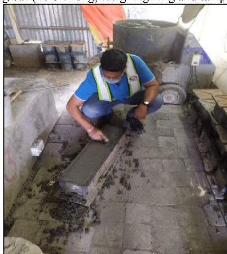
Fig.6 Finishing of Concrete Beam in Concrete Lab
