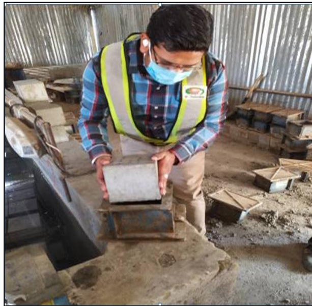
Fig 7. De-moulding of Cubes
