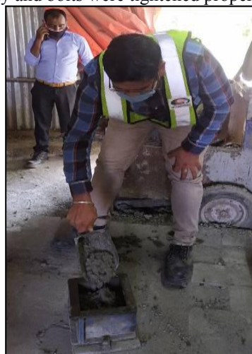
Fig.3 Placing Of Concrete Mix in the Moulds in Concrete Lab
