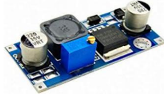
Fig. 2: DC-DC Buck Converter
