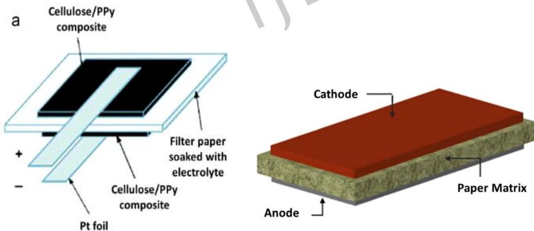
Figure 8 Schematic Diagram of paper battery
