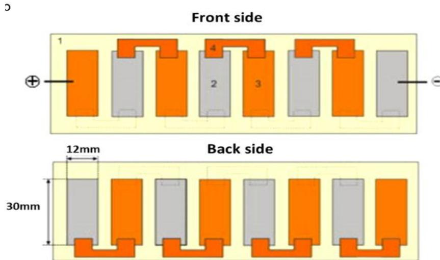
Figure 9. Series integration of cell elements 1) Vegetal-paper, (2) Al anode, (3) Cu cathode, (4) connection
