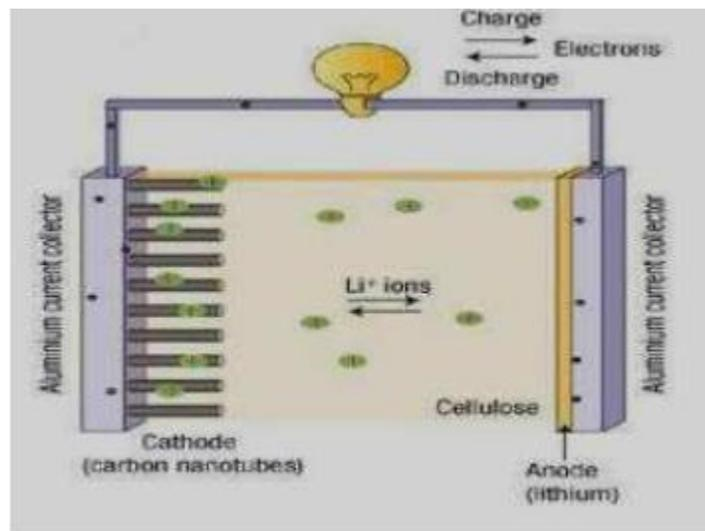
Figure 7 Construction of Paper Battery
