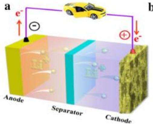
Figure 10. Schematic Diagram of Li-Sulfur Cell
