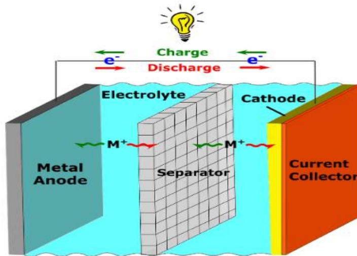
Figure 3. Battery with its components
