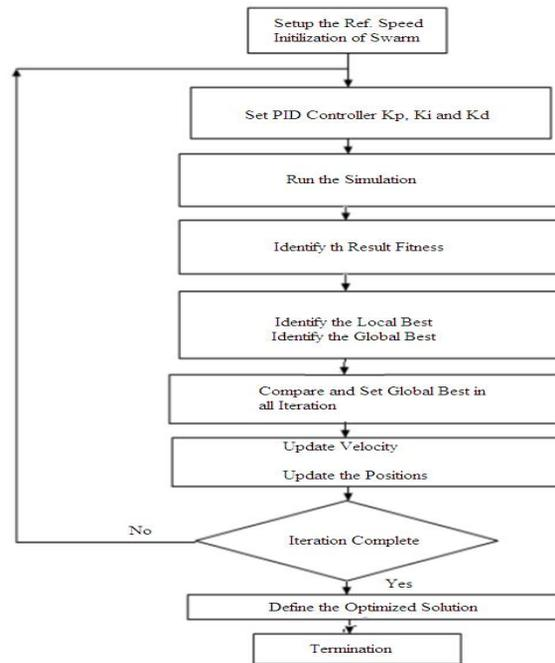
Fig 8. PSO Algorithm for tuning of BLDC Motor Controller
