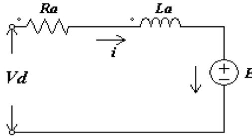
Fig 7. Per Phase equivalent of BLDC motor
