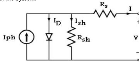
Fig 2. PV cell equivalent circuit
