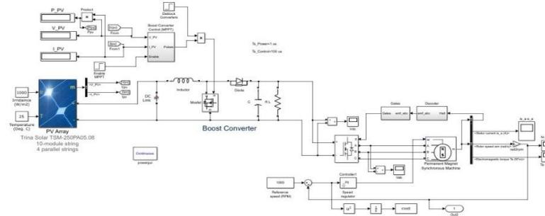
Fig 11. Model of BLDC motor with solar array and ps
