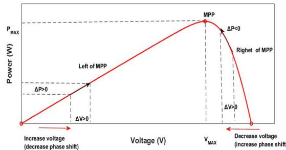
Fig 4. Perturb and Observe on P-V curve
