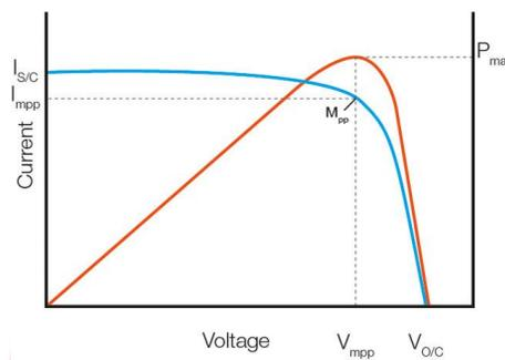
Fig 3. I-V and P-V characteristic of solar array
