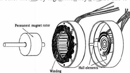
Fig 6. Disassembled view of BLDC motor
