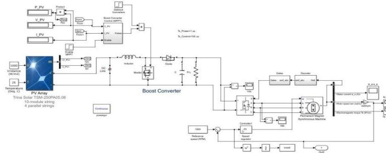
Fig 11. Model of BLDC motor with solar array and psO
