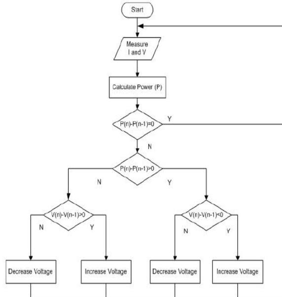
Fig 5. Perturb and Observe flowchart
