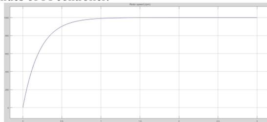
Fig 10. Rotor speed for BLDC motor with solar array
