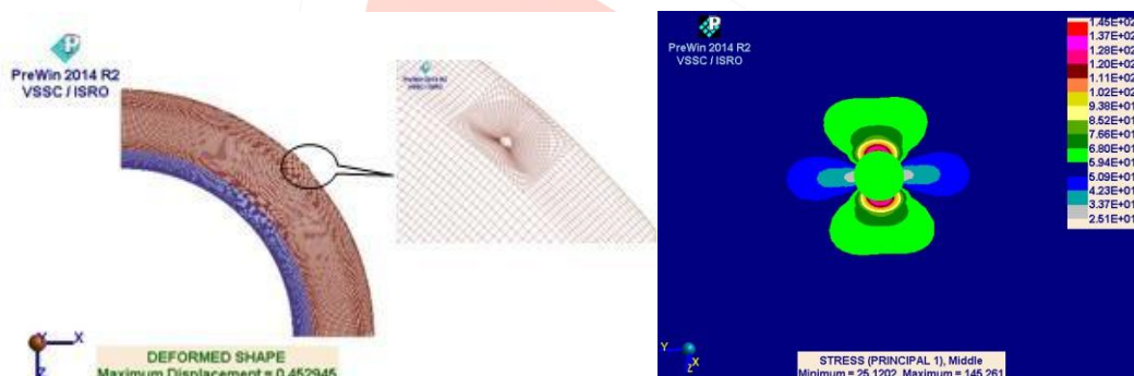
Fig.16: Deformed shape for hole dia.20mm Fig.17: First Principal stress (Mid layer)
