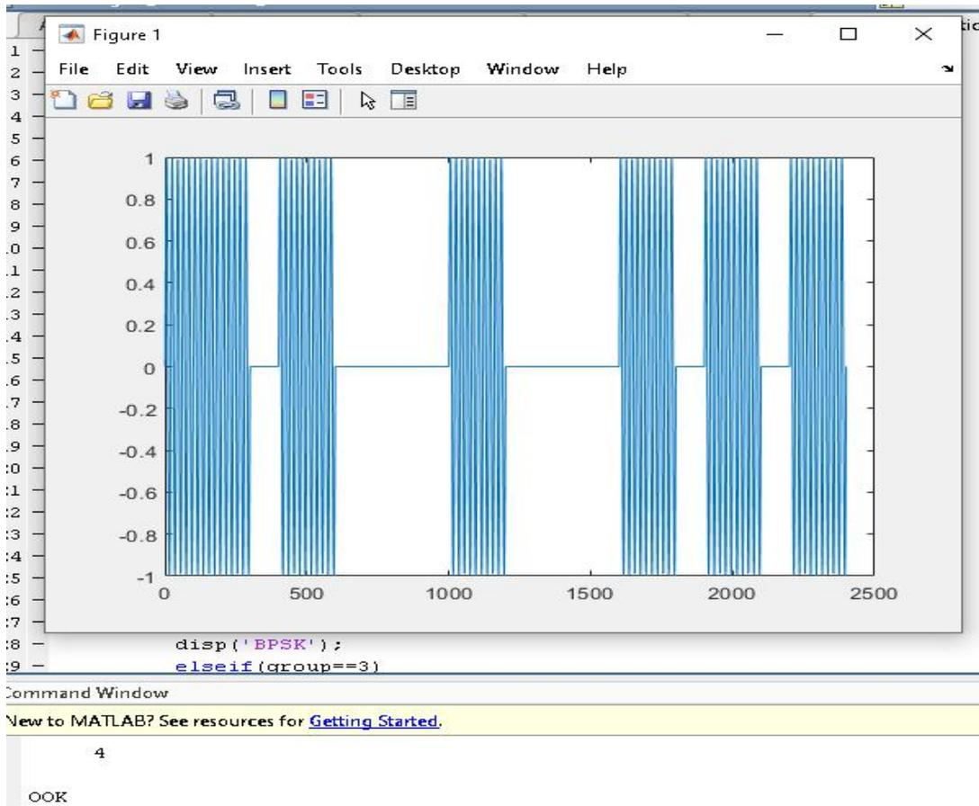
Fig 7: Modulation recognition of digital OOK modulation
