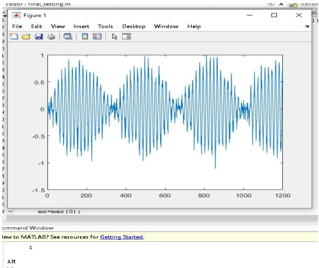
Fig 3: Modulation recognition of analog AM modulation
