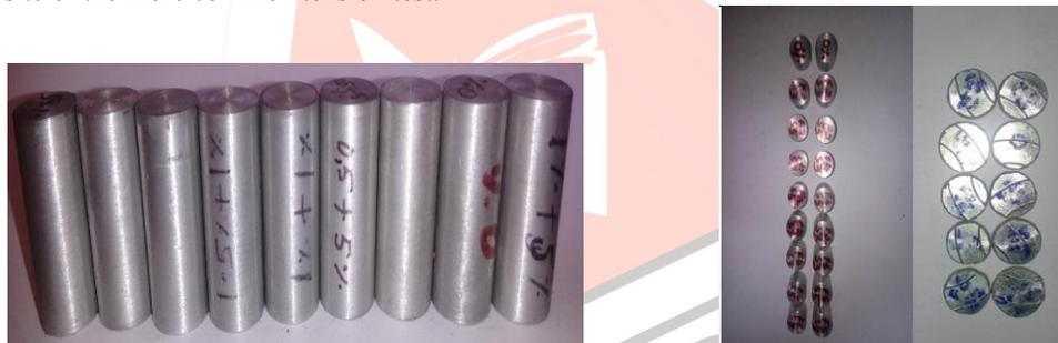
Fig 8: Specimen before Compression test and After test
