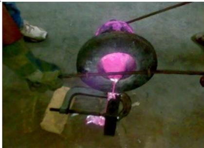
Fig. 4 Pouring of Molten metal into die
