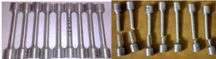
Fig 7: Specimen before and After test
