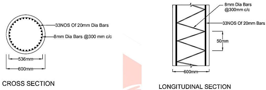
Fig 6: Reinforcement Column details
